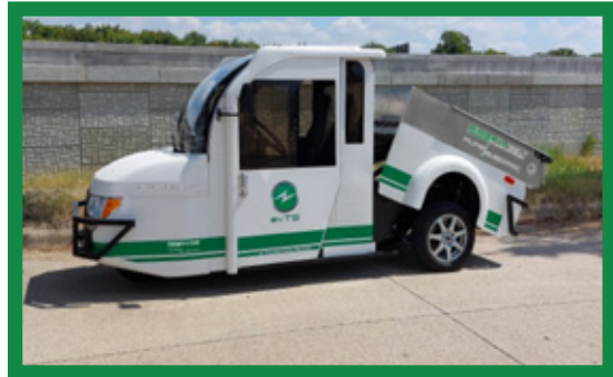
The FireFly has accessory beds for many specialized use cases, like an electric dump
